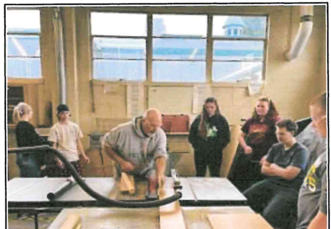
Mr. Carrigan demonstrates the safe procedure for using our SawStop table saw. All students must pass the safety test before using this equipment. (FYI, our insurance underwriter, PACE , help fund the purchase of this saw.)
